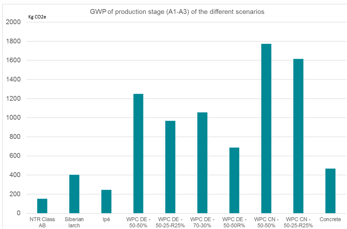
Figure 11. The global warming potential of the different life cycle phases for the different terrace scenarios. The effect of changing the input parameters of the WPC terrace is shown. DE: Germany, CN: China, R: post-consumer recycled polymers. E.g. WPC DE – 50-25-R25% is WPC produced in Germany with 50% wood, 25% polymer (virgin) and 25% post-consumer recycled polymer.
